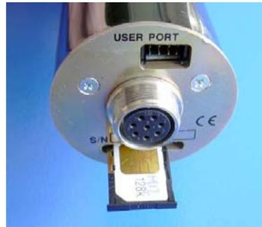
Fig. 4-3 SIM card installation
