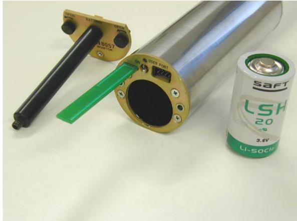
Respect polarity when replacing the battery!
