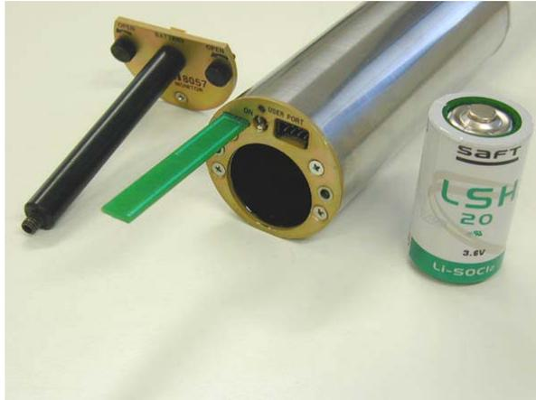
Respect polarity when replacing the battery!
