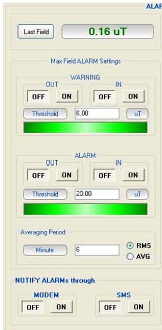
**Fig. 6-5** Last Field, as shown by the control software, and field alarm thresholds settings. Reference on primary probe as default.
