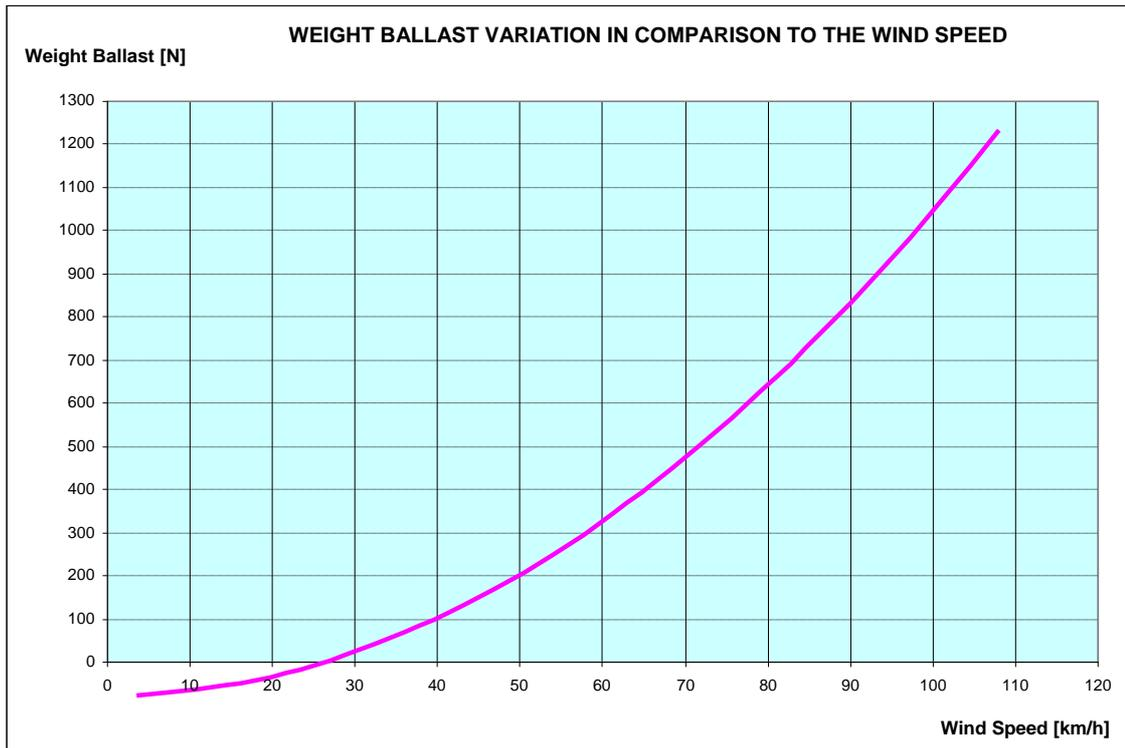
**Fig. 9-4** Weight Ballast variation in comparison to the wind speed for AMB-8057/03 with joint
