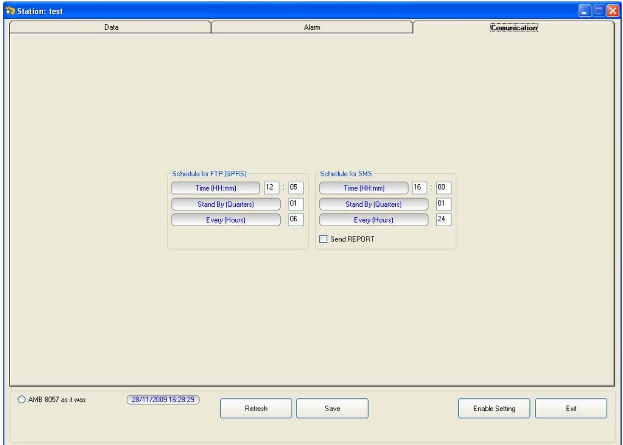
The above example shows that the station modem will switch ON for an FTP connection to the server at 12:05, it will stay ON for 15 minutes (1 quarter). Every 6 hours the loop will be repeated so that the modem will switch ON, and the station will download its data at 12:05, 18:05, 00:05, 06:05 every day. So frequent connections are set for test purpose only, if the parameter **Every (Hours)** was set to 01 the station downloaded its data every hour.
