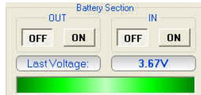
The bar turns red when the value is below the minimum or above the maximum and if the alarm notification is enabled an appropriate message will be sent via SMS.
