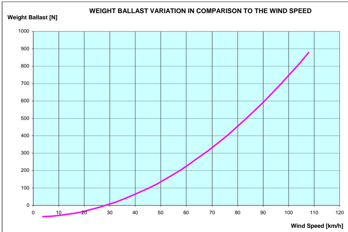
**Fig. 9-3** Weight Ballast variation in comparison to the wind speed for AMB-8057/03 without joint
