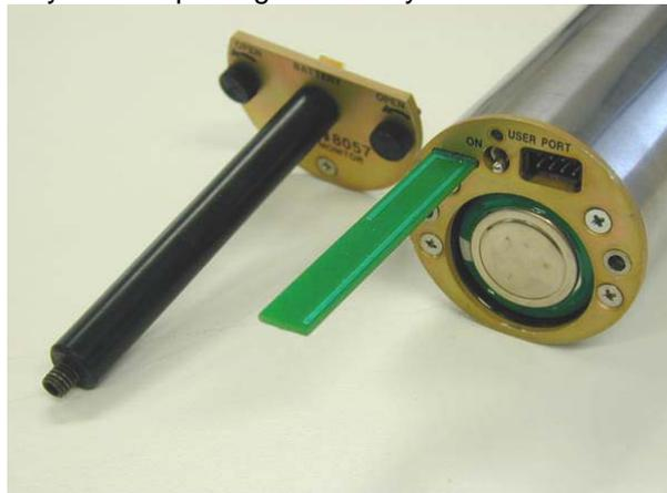
Close the cover of the battery compartment with the thumb screws
