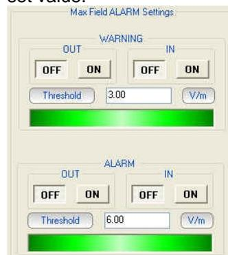
In this example an alarm will occur when the field exceeds 3 or 6 V/m averaged on the time period defined with the option Averaging Period. Thus, brief but intense field variations will not necessarily cause any alarms if the averaged value (in this example on 6 minutes) does not exceed 3 or 6 V/m.
