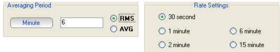
If an Averaging Period of 6min and a rate of 1min are selected the indication will represent, minute by minute, the field average calculated on the previous 6 minutes.
