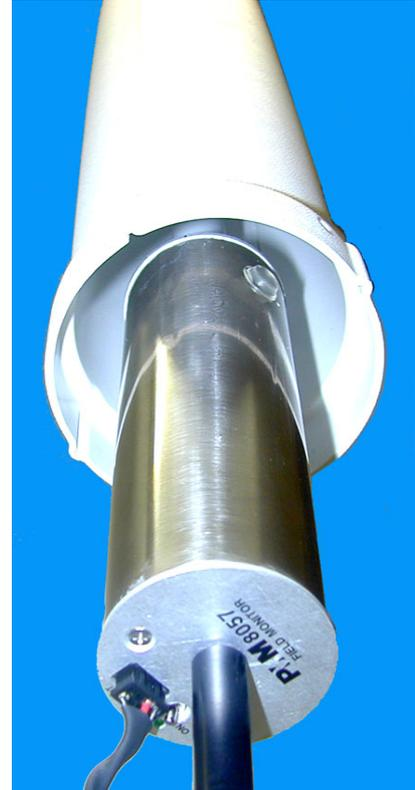
**Fig. 2-5** Removal protective case from 8057/01 and AMB-8057/03
