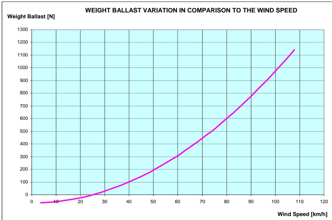
**Fig. 9-2** Weight Ballast variation in comparison to the wind speed for AMB-8057/02 with joint
