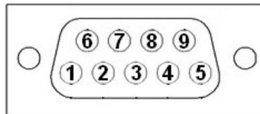
Fig. 1-17 DB9 Female front side view
