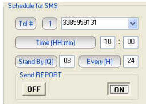
With the **Send REPORT** command **ON**, at the time indicated in the window **Time (HH:mm)** the monitoring station automatically sends its daily report to all the mobile phones listed.
