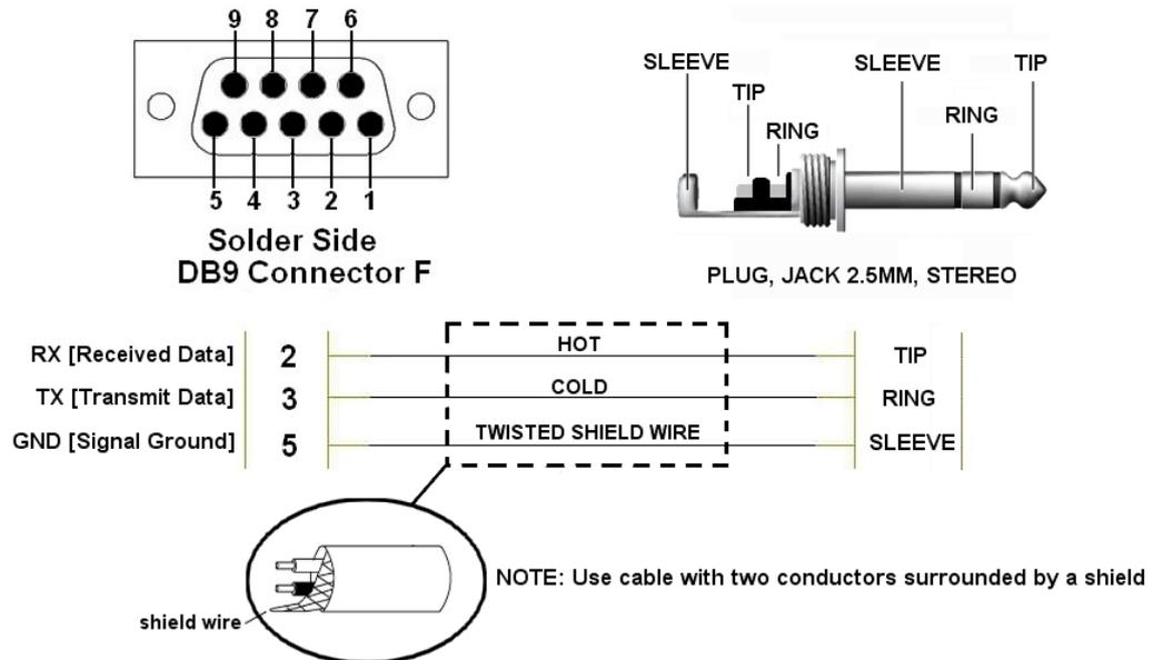
**Fig. 1-12** Serial cable, Jack (m) – DB9 pin configuration
