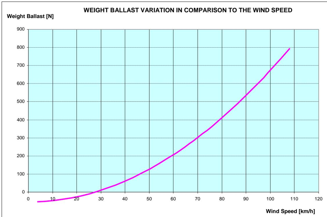
**Fig. 9-1** Weight Ballast variation in comparison to the wind speed for AMB-8057/02 without joint
