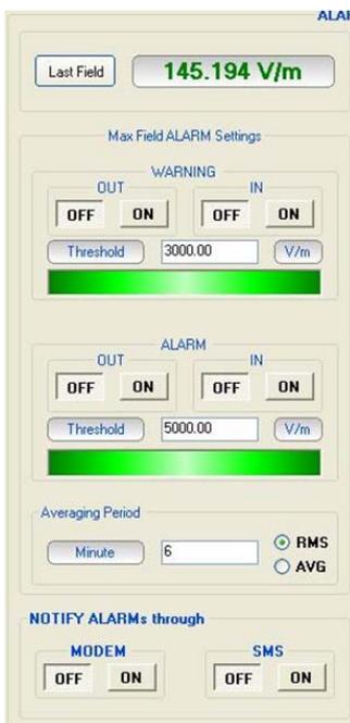
**Fig. 6-6** Last Field, as shown by the control software, and field alarm thresholds settings. Reference on secondary probe.
