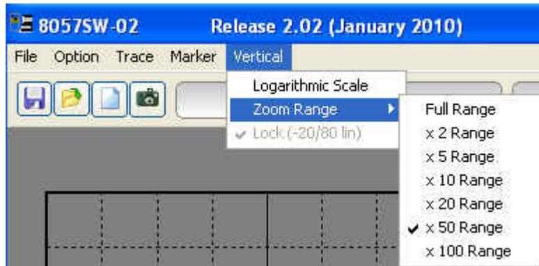
Selecting **x 100 Range** the maximum sensitivity is displayed (scale range equal to 1 V/m).
