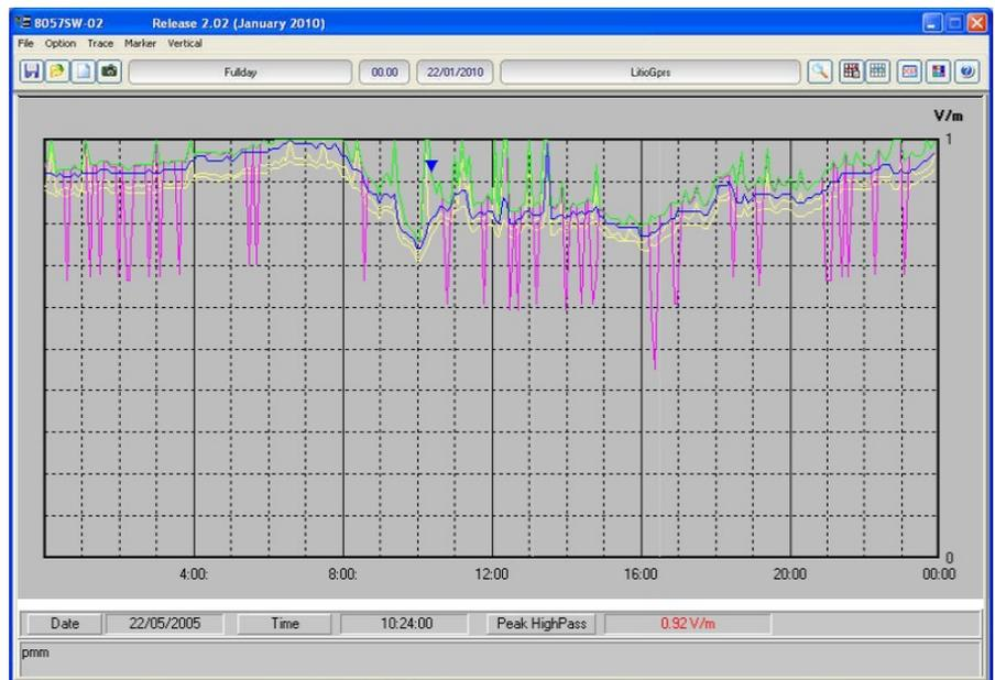
The function **Lock (-20/80 lin)** is activated when the User want to display on the graph both the temperature and the field trace. It forces the scale between -20 and 80 and shows everything in linear mode.
