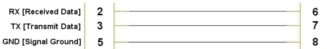
**Fig. 1-11 AMB-8057/02 Serial cable pin configuration for User Port**
