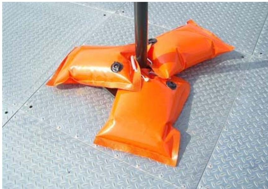
Fasten the ballast bags to the mast using the plastic straps.
