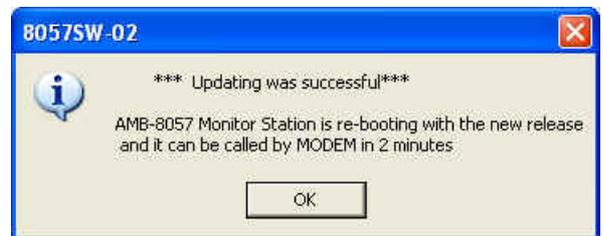
If any CRC errors occur or if, in CSD mode, there is a poor telephone connection, or if for any reasons the new firmware is not completely and successfully transferred to the monitoring station, the station will automatically restore the old firmware in order to prevent malfunctions or stops.
